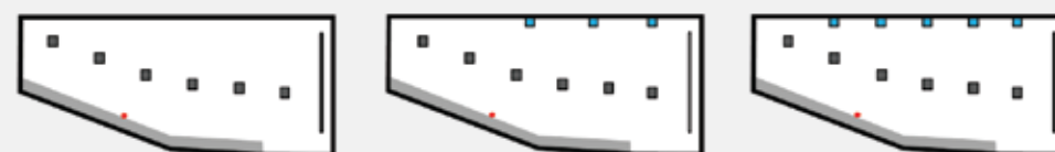
Side views showing side wall speaker options for cinemas that include ceiling speakers
